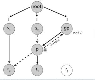
→ The INDEP fault-tolerance protocol
